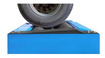
The heavy brake tester is lifted by **hydraulic cylinders**. An oil-hydraulic circuit with flow dividers allows the frames to be lifted **synchronously**.
